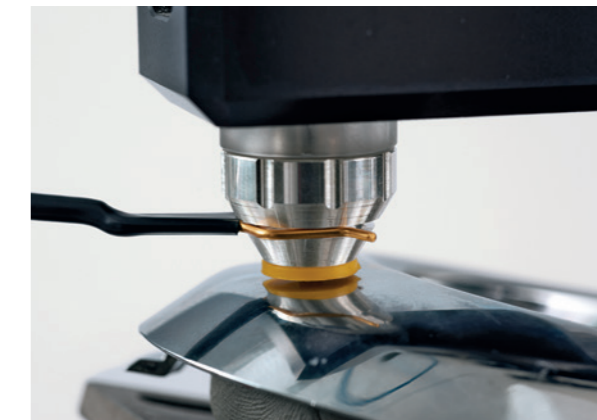
STEP Test measuring cell placed on a specimen
