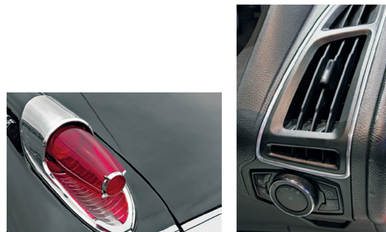
Typical application for the CMS2 STEP: chrome-plated trim elements in automotive manufacturing, based on multiplex nickel coatings
