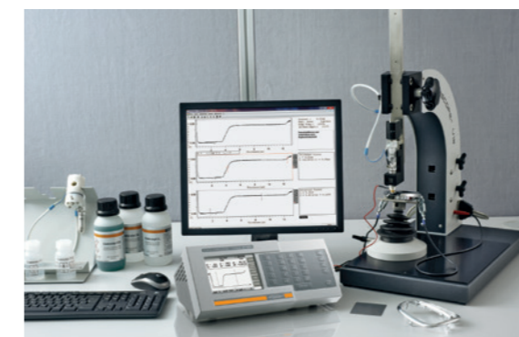
COULOSCOPE CMS2 STEP workstation: Support stand V18 with ball-jointed sample support and swivelling clamping plate. The measuring cell storage rack for stowing the measuring cell can also hold up to three 100-ml laboratory bottles
