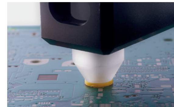
Measuring the thickness of remaining tin on a printed circuit board
